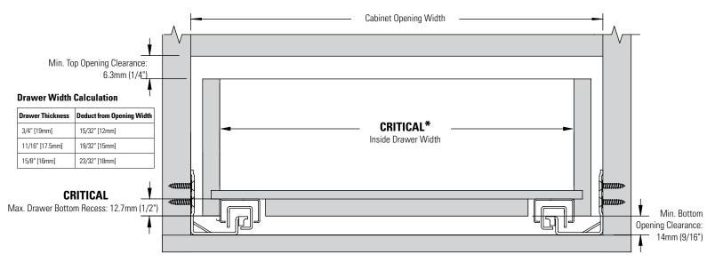
\*Cabinet Opening Width Minus 50mm (1-31/32") = Inside Drawer Width MuV Maximum Drawer Side Material Thickness: 19mm (3/4")
