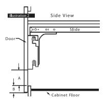
**Step 6:** Hang door with brackets attached on the mounting screws on to the product members. Tighten bottom screws securely. Tighten top screws (with washer) snugly allowing for future adjustment. (See illustration 5.)
