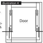
**Step 2:** Measure the distance from the bottom face frame to bottom of the Door Bracket. **Note as Dimension A.** Measure your door overlap. **Note as Dimension B.** (**See illustration 2**) **Note:** On frameless cabinets, measure from the bottom of the cabinet opening to the bottom of the Door Bracket.
