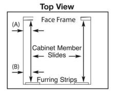
**Step 5:** Mount Rear Bracket. Extend the slide rear mounting bracket until it contacts the rear (Furring Strip). Bottom of slide should be (13 \( \frac{13}{9} \) '' - 35 \( \& \) 27Qt. 19" - 50Qt.) from cabinet floor. Rear mounting bracket should be the same distance from the side cabinet wall at rear of slide as it is up front. Drive mounting screw in center horizontal slot of rear mounting bracket, tighten. Tighten screw in front bracket.
