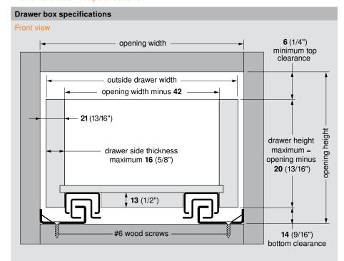
NOTE: Drawer side material thickness may vary. Precise measurement of drawer side material thickness should be used when calculating outside drawer width using the table below. Inside drawer width **must** equal opening width minus **42** (1-21/32") for TANDEM to align and function optimally.
